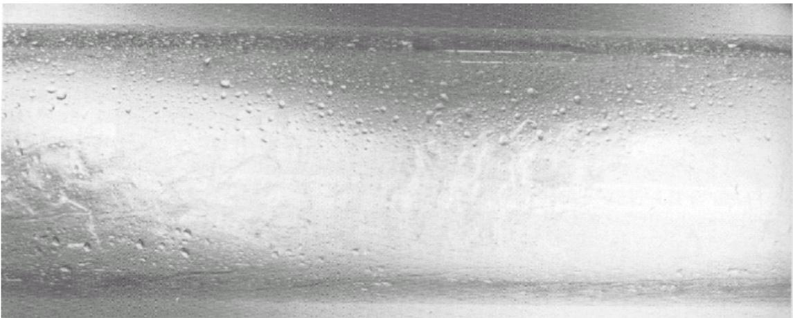
Figure 2-12: Stratified flow with the deposited droplets at the top
