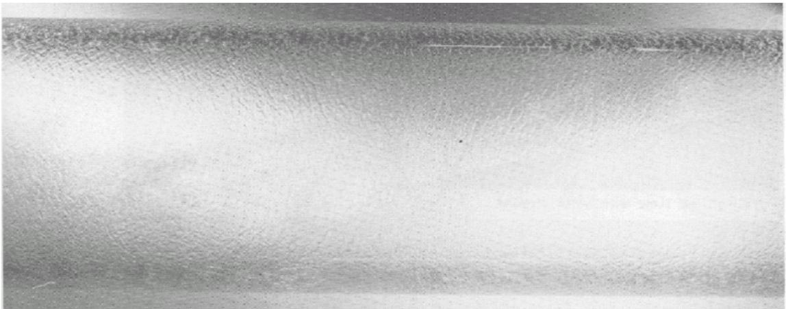
Figure 2-14: Annular flow ( $ID = 9.53\text{cm}$ ,  $U_{SG} = 31\text{ m/s}$ , and  $U_{SL} = 0.076\text{ m/s}$ )
